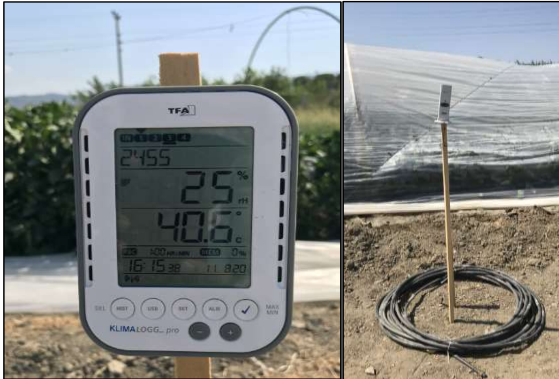
Figure 5. Data logger and wireless transmitter used to record temperature values during heat stress.
